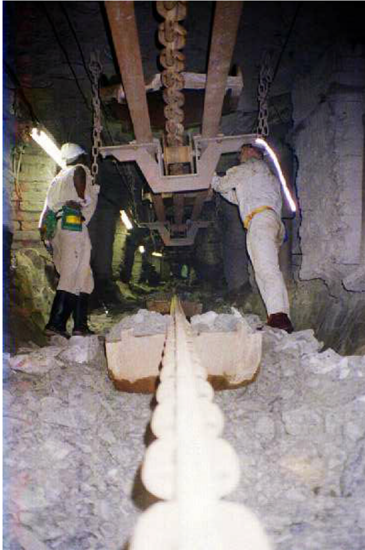
Figure 1.19 Up-dip continuous scraping facility currently on trial in a deep CSDP stope.
